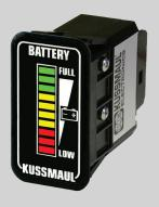
The Mini Single Bar Graph Display 091-234 is a universal display containing a 10-LED bar graph to indicate the vehicle's battery status. The top or bottom LED's blink to indicate HIGH VOLTAGE or LOW VOLTAGE is detected. respectively. The switch is designed to fit into a standard 1.45" x 0.83" panel cut-out.
