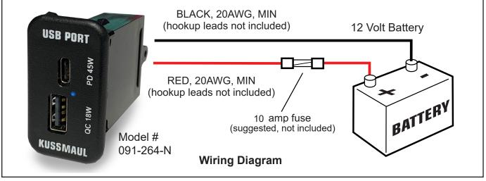
**Current Limit Protection** - Each output of the USB charger is automatically current limited to approximately 3 Amps during overload and short-circuit conditions. During this condition, the LED will be extinguished. If an overload or fault condition is suspected, immediately disconnect all connected USB devices. The LED will illuminate and the outputs will return to normal operation as soon as the overload or fault condition is corrected.
