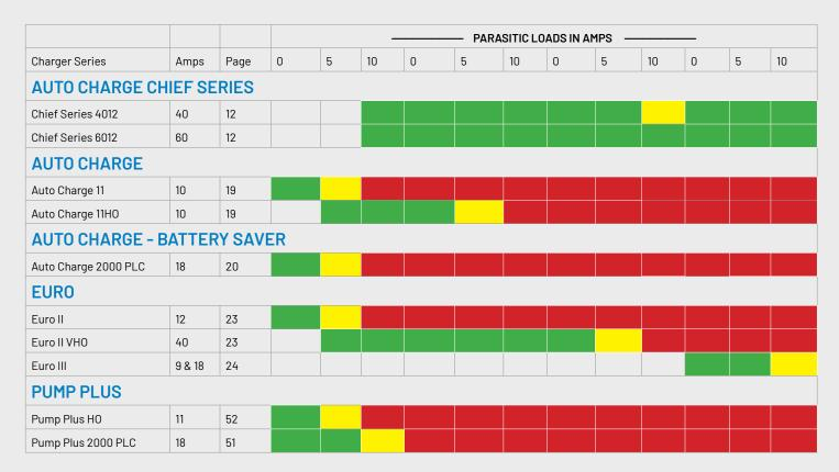
These chargers are for average recharge rates and average sized batteries. For specific applications, please contact our sales or engineering department with battery size, parasitic loads and required recharge time.
