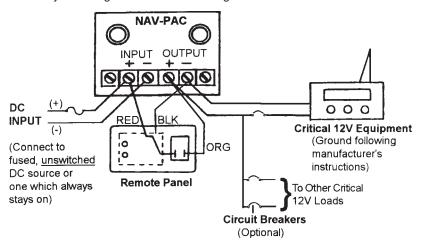
Remote Panel: Mount in a conspicuous location where the loss of power indication will be noticed. The NAV-PAC will function normally without the remote panel or with the remote panel switch off. Connect the wiring as follows: (see diagram)
