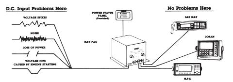
The NAV-PAC protects electronics from voltage spikes, power surges, momentary power losses, abrupt voltage changes and noise interference on incoming DC power to MDTs, GPS, CHART PLOTTERS and other Onbaord Electronics prone to memory loss or "crashes".
