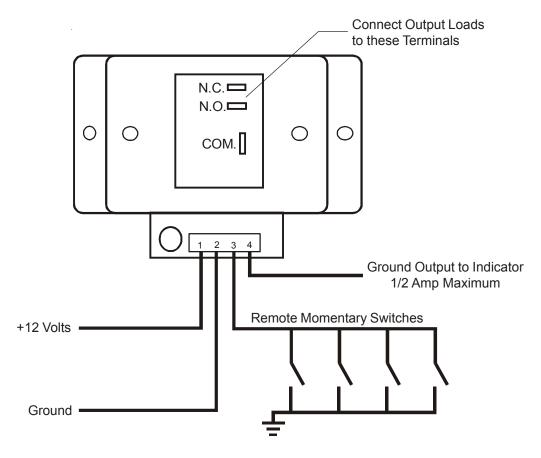
**Note**: To retain relay position memory connect +12 Volts directly to the battery. To reset relay on startup, connect +12 Volts downstream of master switch. LED Illuminates when output relay is energized.
