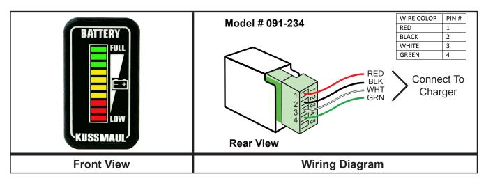
**High/Low Voltage Alert -** The Mini Single Bar Graph Display contains detection for when there is a high or low voltage in the vehicle battery. Knowing when the vehicle's battery voltage is too high or low can help to protect the battery, and extend its life through proper use and maintenance. When there is HIGH VOLTAGE the top LED will blink. When there is LOW VOLTAGE the bottom LED will blink.
