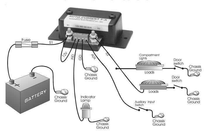
The Auto Current F-A detects current and closes a switch when the sensed current flows, to provide a remote indication. An electronic frasher interrupts the indicator output approximately once per second to provide a flashing indication.
