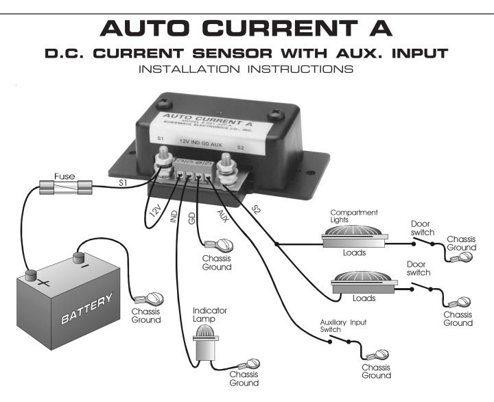
The Auto Current A detects current and closes a switch when the sensed current flows, to provide a remote indication. The current detected may be from compartment lights as illustrated or from any other D.C. Load in the range.
