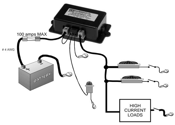
The Auto Current detects current and closes a switch when the sensed current flows, to provide a remote indication. Designed for applications where a remote indicator must be illuminated when one or more lights or other loads are energized. By detecting load current any one, or more than one lamp, or other load will cause the indicator to light. The indicator circuit contains a relay which is operated by the sensor, indicator currents as high as 5 amperes may be driven by relay.
