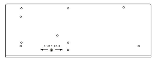
Use a mini precision slotted screwdriver to select AGM or Lead-Acid
