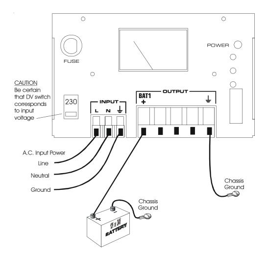
**IMPORTANT**: Charger output wire size is AWG #8, minimum. Wire size is for a maximum length of 20 feet. If wiring is to be longer, larger wiring is required. Additional information is available on request.
