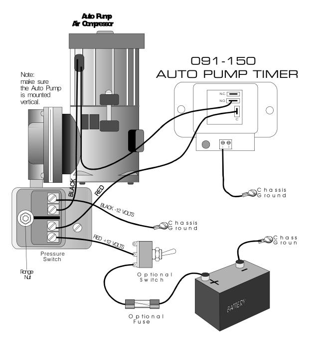
**CAUTION:** Observe correct polarity connections Red lead to motor and timer **MUST** be positive
