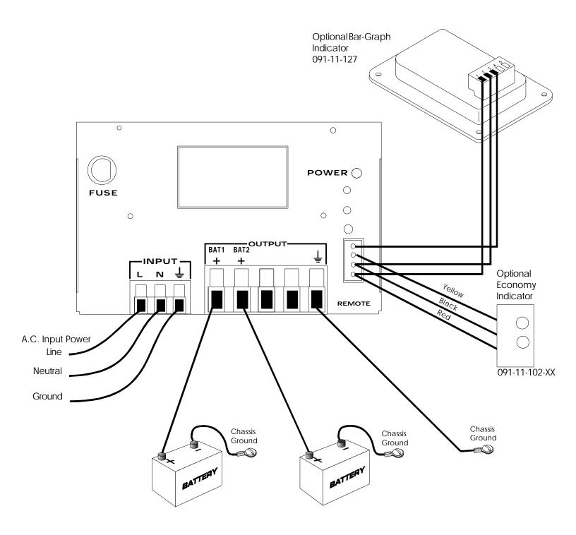
**IMPORTANT**: Charger output wire size is 12 awg. Wire size is for a maximum length of 20 feet. If wiring is to be longer, larger wiring is required. Additional information is available on request.
