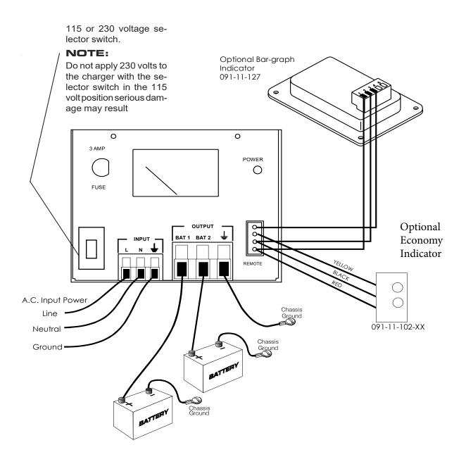
**IMPORTANT**: Charger output wire size is 14 awg. Wire size is for a maximum length of 20 feet. If wiring is to be longer, larger wiring is required. Additional information is available on request.
