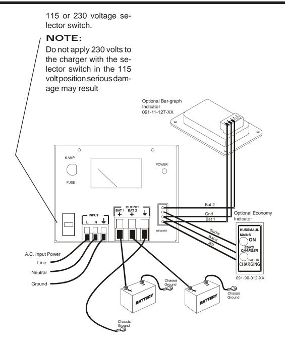
**IMPORTANT**: Charger output wire size is 14 awg. Wire size is for a maximum length of 20 feet. If wiring is to be longer, larger wiring is required. Additional information is available on request.
