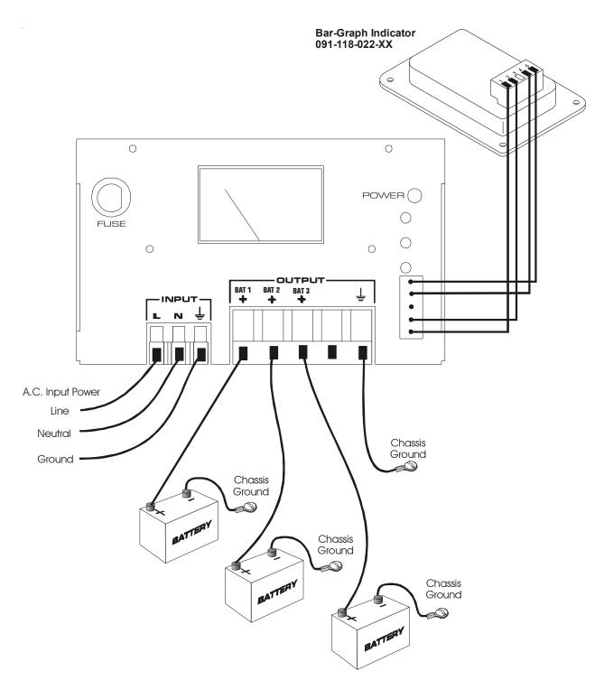
**IMPORTANT**: Charger output wire size is 12 awg. Wire size is for a maximum length of 20 feet. If wiring is to be longer, larger wiring is required. Additional information is available on request.
