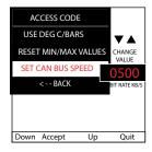
Serial #'s starting with the letter 'B' can be adjusted to various Can Bus Bit Rates: 50,125,250,500,1000 K Bits. Units are factory set to 500K.
